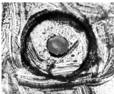
Figure 30 Damage from improper cleaning.
